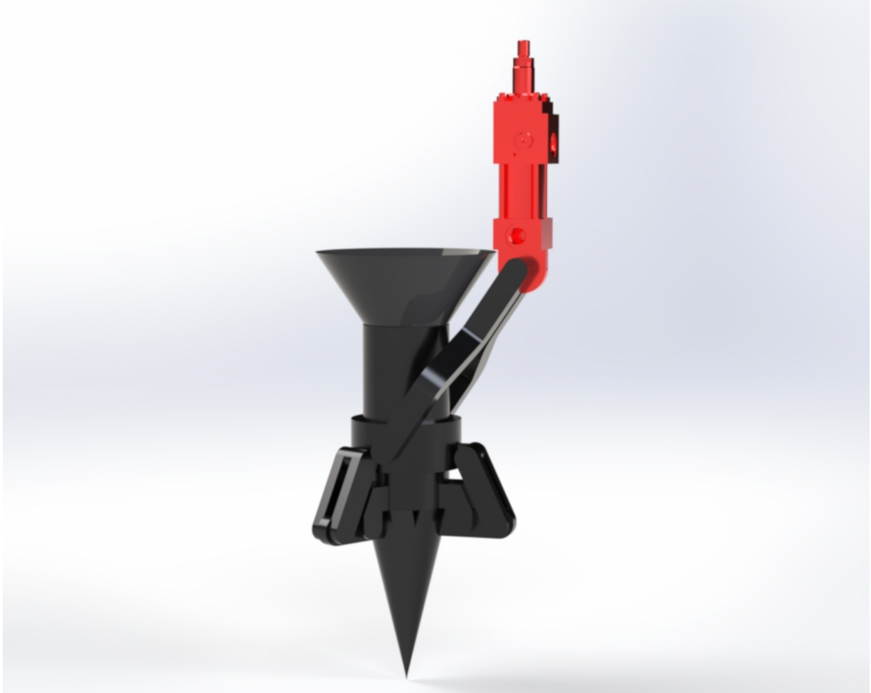
Figure 9: Planter and hydraulic cylinder with toggle linkage mechanism
