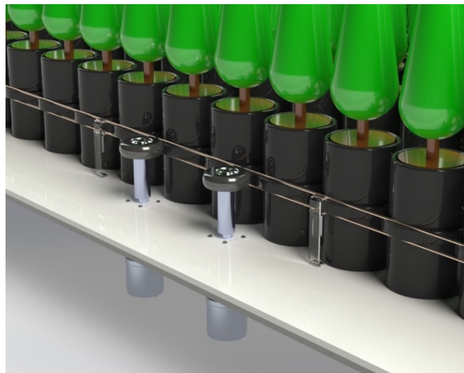
Figure 6: Close-up View of Sapling Pucks and Drive Mechanism
