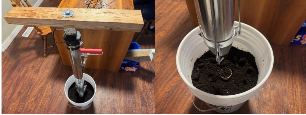
Figure 18: Load cell testing setup for sapling insertion force measurement
